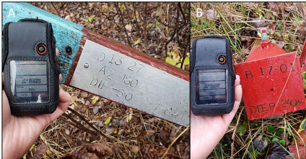
Figure 12.2: Examples of Onsite Collar Location Verification (A) D13-27 collar; (B) B17-01 Collar
