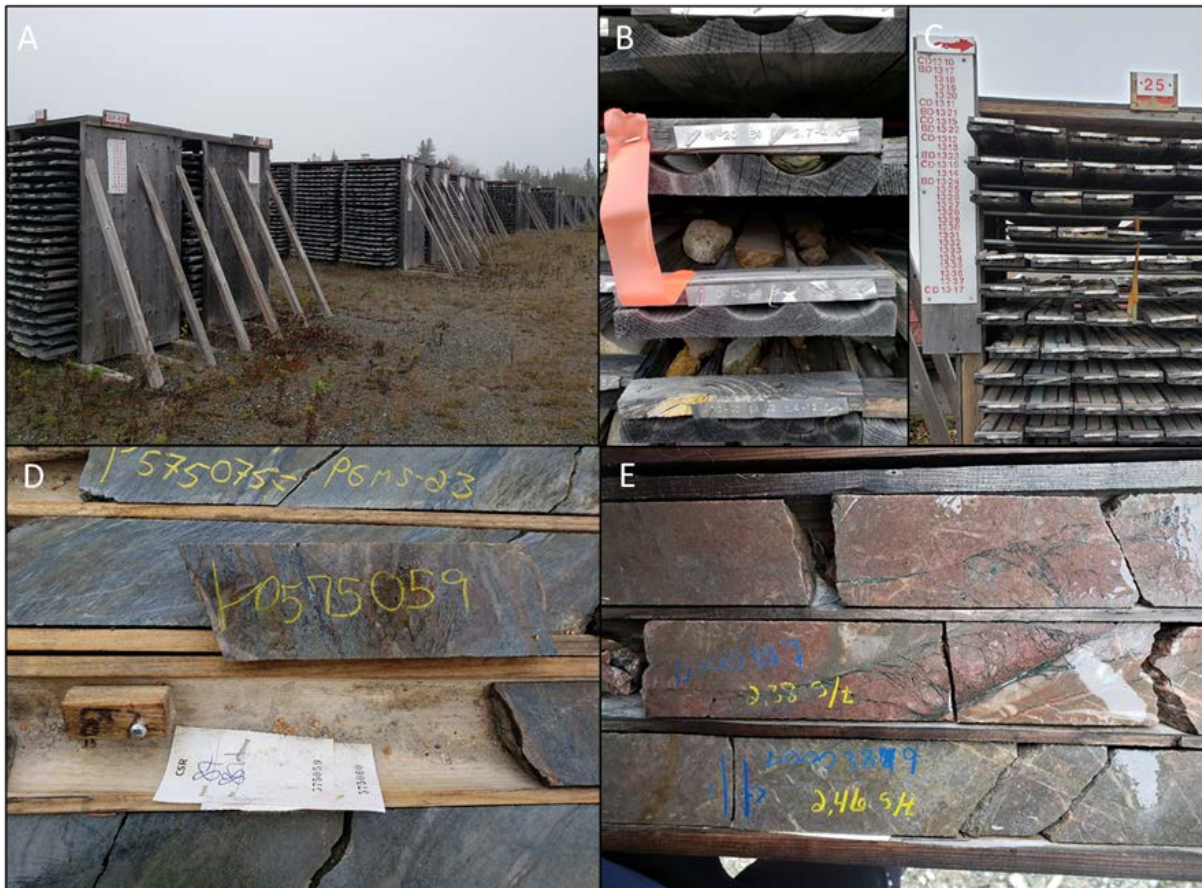
A) Core racks; B and C) Proper labelling of the core racks and drill core boxes; D) Sample tag stapled in the core box; E) Mineralization in hole BD10 117
